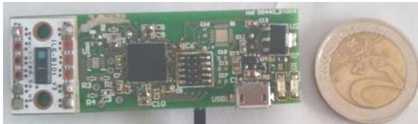
Figure 3. Prototype based on the QFN68 package of PSoC5 LP by Cypress Semiconductor Corp.
