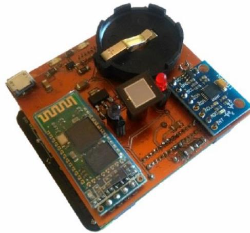
Figure 2. Initial prototype based on the CY8CKIT-001 development kit by Cypress Semiconductor Corp.
